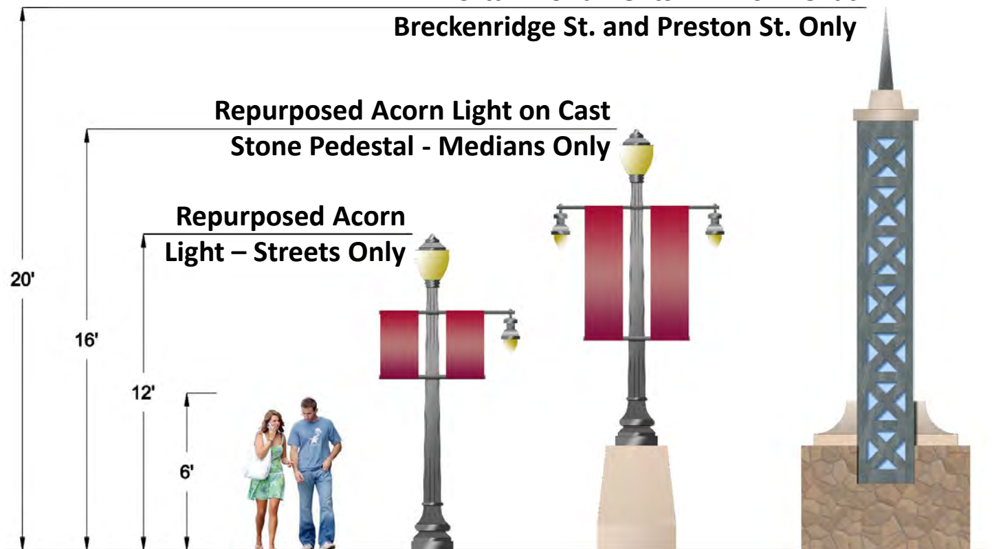
Figure 88. Repurposed Acorn Light Fixtures
